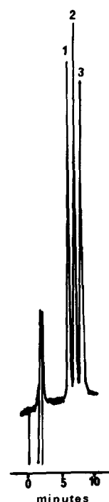
FIG. 2. High performance liquid chromatogram for \alpha, \gamma and \delta tocopherols assays. 1 : \delta -tocopherol; 2 : \gamma -tocopherol; 3 : \alpha -tocopherol.
